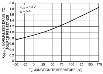
Figure 5. On–Resistance Variation with Temperature
