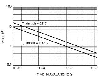
Figure 12. I<sub>PEAK</sub> vs. Time in Avalanche
