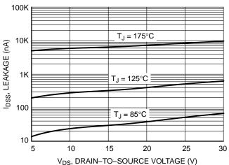
Figure 6. Drain-to-Source Leakage Current vs. Voltage
