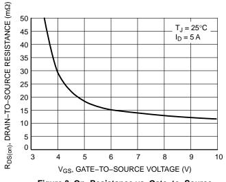
Figure 3. On-Resistance vs. Gate-to-Source Voltage
