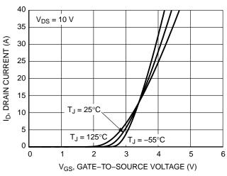
Figure 2. Transfer Characteristics
