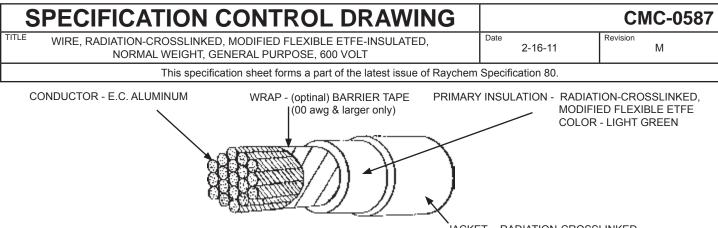
JACKET - RADIATION-CROSSLINKED, MODIFIED FLEXIBLE ETFE
