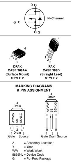
\* The Assembly Location code (A) is front side optional. In cases where the Assembly Location is stamped in the package, the front side assembly code may be blank.
