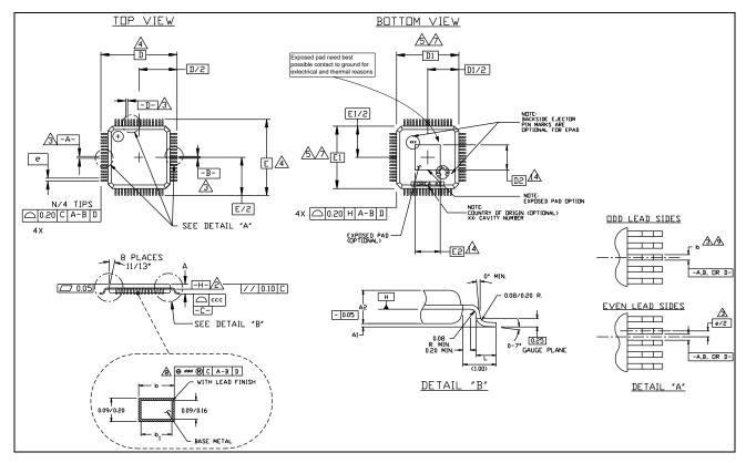
Figure 6 - TQFP 7x7 Drawing
