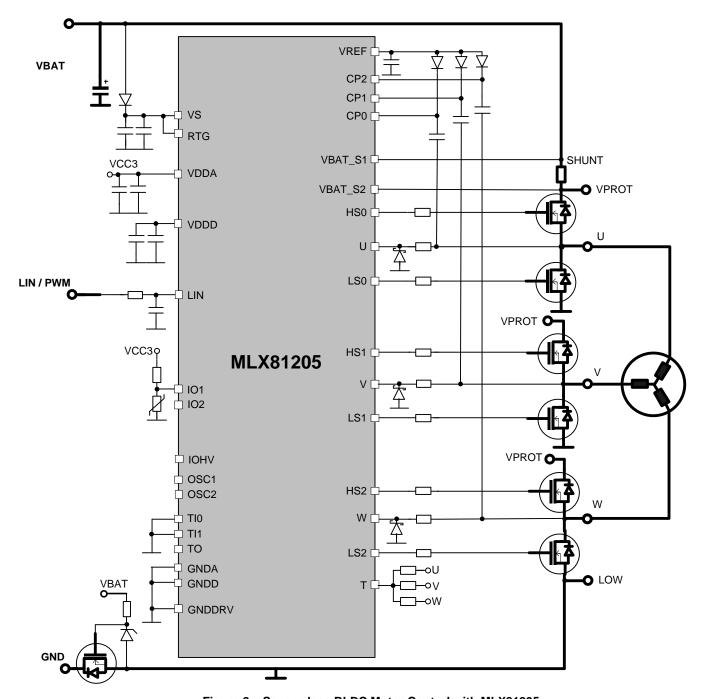
Figure 2 – Sensor-less BLDC Motor Control with MLX81205
