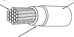
PRIMARY INSULATION - RADIATION-CROSSLINKED, MODIFIED FLEXIBLE ETFE **COLOR - LIGHT GREEN**
