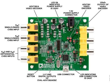
Figure 3. ADV7282A Evaluation Board
