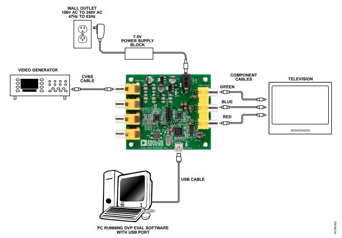
Figure 2. Outline of Evaluation Board Connections
